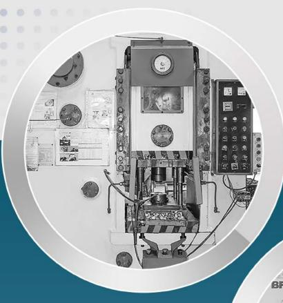
Parts weighing between 70g-1500g can be forged using our mechanical and hydraulic presses ranging from 50T - 450 T.
